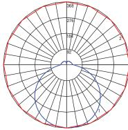
Maximum Candela = 367.53 Located At Horizontal Angle = 315, Vertical Angle = 3 # 1 - Vertical Plane Through Horizontal Angles (315 - 135) (Through Max. Cd.)
