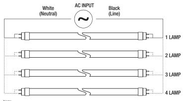
Note: 1. LEDlescent<sup>™</sup> lamp is polarity neutral. Can be installed in either direction. 2. Sockets may be shunted or non-shunted. Tie socket leads together for non-shunted sockets.
