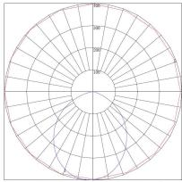
Maximum Candela = 400.13 Located At Horizontal Angle = 157.5, Vertical Angle = 4 # 1 - Vertical Plane Through Horizontal Angles (157.5 - 337.5) (Through Max. Cd.) # 2 - Horizontal Cone Through Vertical Angle (4) (Through Max. Cd.)
