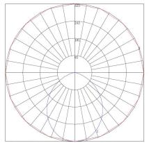
Maximum Candela = 322.82 Located At Horizontal Angle = 90, Vertical Angle = 1 # 1 - Vertical Plane Through Horizontal Angles (90 - 270) (Through Max. Cd.) # 2 - Horizontal Cone Through Vertical Angle (1) (Through Max. Cd.)
