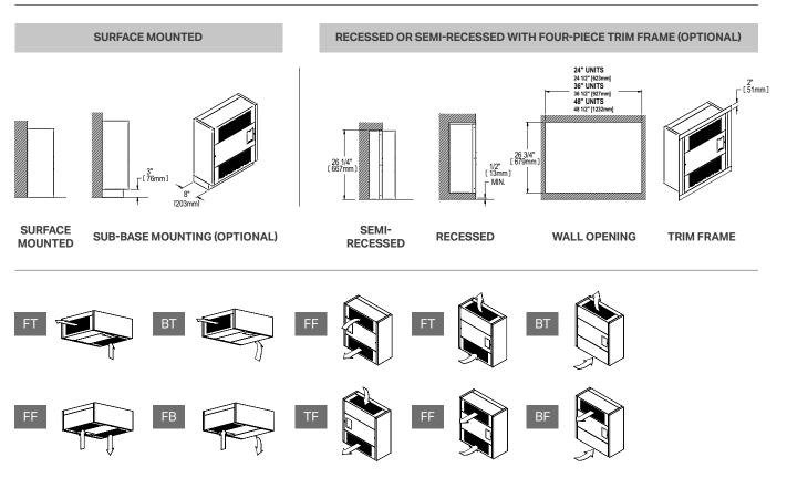
SEVERAL AIRFLOW CONFIGURATIONS ARE POSSIBLE AND ADAPTABLE ON CONSTRUCTION SITE: F = FRONT, T = TOP, B = BOTTOM
