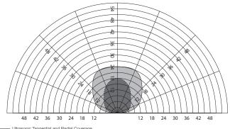
Ultrasonic Tangential and Radial Coverage
