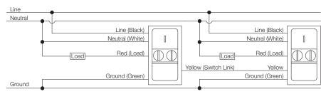
VS 1 (Master / Auxiliary) Three-way Wiring - up to maximum 4 sensors can be grouped via "Switch Link"
