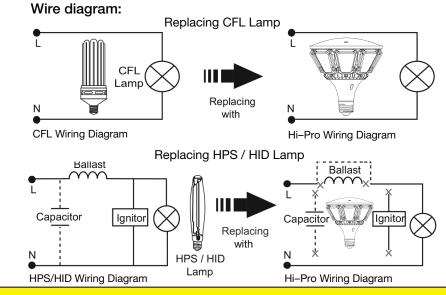
Warning: Disable all power to the Luminaire. The lamp holder must be disconnected from the wiring to the ballast, capacitor, or ignitor. Verify that voltage does not exceed 277V AC. Please see "Wiring Diagram". Failure to follow instructions can result in a damaged product and will void warranty. It could also result in an electric shock, or fire.
