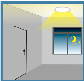
No motion detected, the lamp remains at a low light level all the time.
