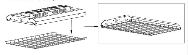
2. Fit the 4pcs buckle into the wire guard, please note that the buckle hole position is flush with the light body.
