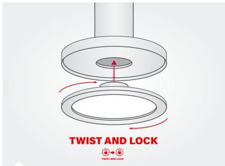
**STEP 3:** ☉ Align the arrow sign ▼ from pendant kit to unlock-sign ☒ from fixture.
