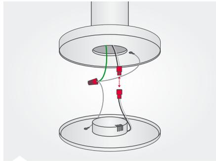
**STEP 2:** Make ground connection. Next simply „click“ the two sides of the orange wire connector together.
