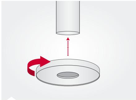
**STEP 1:** Align threads from pipe of pendant kit to mounting bracket. Turn clockwise and lock pipe on mounting bracket.
