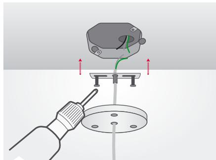
**STEP 4:** Attach the bracket to junction box using the 2 screws (provided). Pull the AC cables through the bracket center hole.
