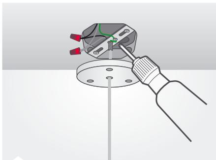
**STEP 5:** Attach connector (provided) to AC cable from junction box: L side to Black side wire. N side to White AC wire.
