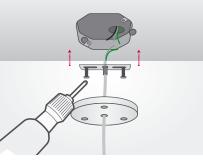
STEP 4: Attach the bracket to junction box using the 2 screws (provided). Pull the AC cables through the bracket center hole.
