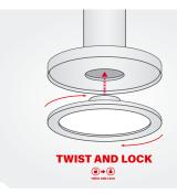
STEP 3: <sup>®</sup> Align the arrow sign ▼ from pendant kit to unlock-sign a from fixture. I Turn clockwise to locked-sign ■ to lock fixture in place. Remove label.
