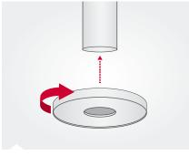
STEP 1: Align threads from pipe of pendent kit to mounting bracket. Turn clockwise and lock pipe on mounting bracket.
