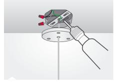
STEP 5: Attach connector (provided) to AC cable from junction box: L side to Black side wire. N side to White AC wire.
