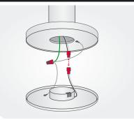
STEP 2: Make ground connection. Next simply "click" the two sides of the orange wire connector together.
