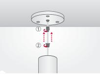
STEP 6: Push and feed all wires up into junction box as you raise the cover plate into place. Tighten the 2 nuts (provided) one by one.
