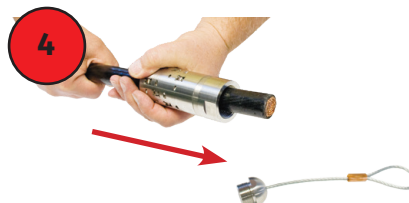
4 Push electrical wire thru Wire Snagger to release it from the tool.
