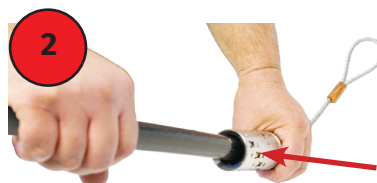
2 Push cable into the tool until it reaches the bottom of the cap, then pull back to make sure the wire is set.
