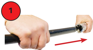
1 Insert electrical wire into Wire Snagger tool body.
