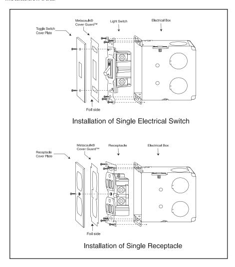
**Step 1** Place aluminum foil side of Metacaulk Cover Guard against inside of electrical face plate.
