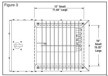
Systems) or Canadian equivalent. Every PRH model is equipped with an inlet and outlet grille for free-air discharge. Both grilles are intended to be removed when connecting to a duct system. The inlet and outlet ends of the unit are equipped with perforated flanges to aid in forming both inlet and outlet duct flanges (see Figure 3).
