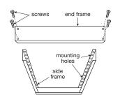
Frame construction for surface mount panels
