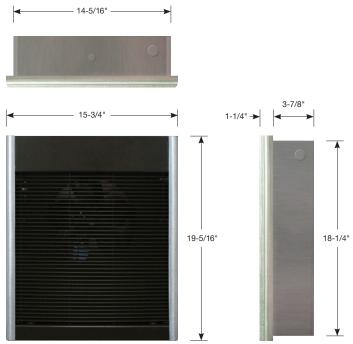
NOTE: \* Will accommodate pneumatic/electric or low-voltage controls commonly used with computerized energy management systems Mounting Limitations: For wall mounting, do not install back box closer than 8 in. from floor or adjacent wall. Do not install heater behind towel rack, behind door, in floor, in closet, in ceiling or where air flow may be obstructed. All controls are concealed behind the front cover making them essentially tamper proof.
