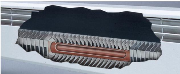
The electric heating element is partially submerged in an inert heat transfer fluid totally sealed in a large 7/8" diameter copper tube spanning the length of the heater. This thermal mass transfers heat evenly across the entire length of the heater. The PLF series provides uniform warmth with longer heat retention and minimal temperature variation.
