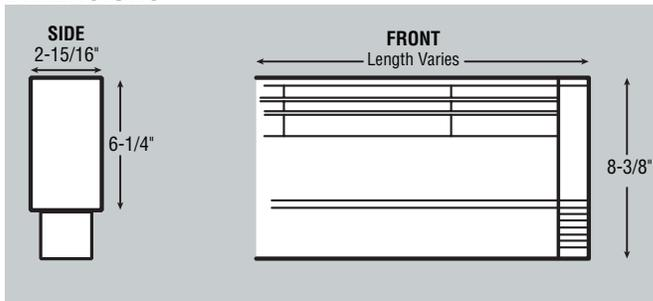
All knockouts are 7/8" diameter for 1/2" conduit
