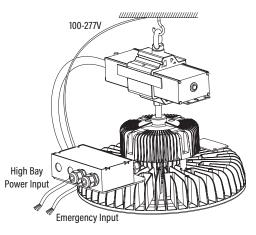
3. Connect the electrical cables; Black-L, White-N, Yellow/Green-Ground. If using in wet locations, ensure all electrical connections and installation holes have a water tight seal.
