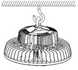
2. Secure hook to the ceiling and hang the fixture from the hook.
