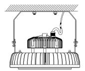
2. Connect the electrical cables. Brown-L, Blue-N, Yellow/Green-Ground. If using in wet locations, ensure all electrical connections and installation holes have a water tight seal.
