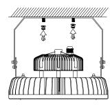
1. Attach the bracket to the mounting surface.
