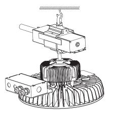
2. Secure hook to the ceiling and hang the fixture from the hook.
