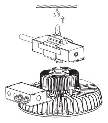
1. Drill a hole into the ceiling for the appropriate size hook (provided by installer).
