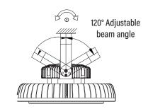
3. Adjust the bracket to the beam angle you need.
