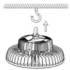
1. Drill a hole into the ceiling for the appropriate size hook (provided by installer).
