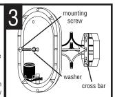
POSITION THE FIXTURE over the outlet box and secure in place with the mounting screw (1/4-20 x 1.1 provided). Screw lamp into lampholder. Use lamp type and wattage specified on
