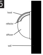
ON MODELS WITH HOOD, attach to wall with reflector up. Hood is to be placed above reflector as shown.
