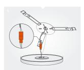
Make wire connections between fixture and junction box connect wires to AC cables from junction box with wire nuts ( provided ): L side to Black AC wire, W side to White AC wire.
