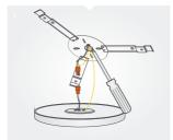
Use M4 screw to install ground from the grid(AC) and from fixture, to the bracket.
