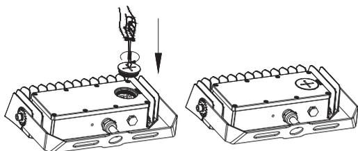
Step 4 : Screw the plug back into the power supply cover plate with a screwdriver.
