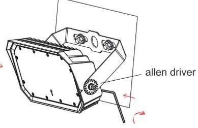
Fasten the screw both sides with allen driver.
