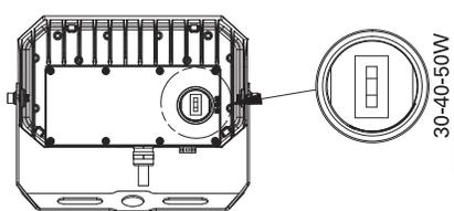
Step 3 : Set power switch to the corresponding position as required;
