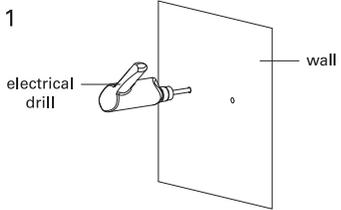
Mark the position of the fixing holes with flood light bracket, then drill the fixing holes.
