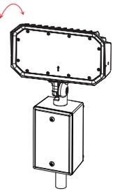
Adjust the lamp into suitable angle.
