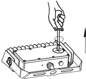
Step 1 : Turn the light-emitting side of the lamp downward and twist out the plug with a cross screwdriver;
