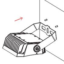
Make the bracket face tightly to the wall through the thread.
