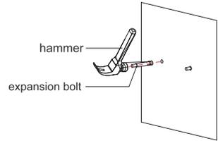
Drive in the bolts to the pre-drilled holes with thread outside, as the below pic indicate.
