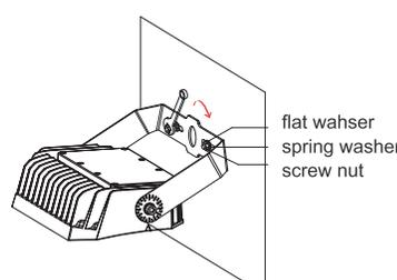
Fasten the screw nut clockwise with provided hardware by wrench.
