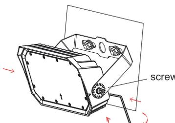
Rotate the light to the proper angle and fasten the screws.
