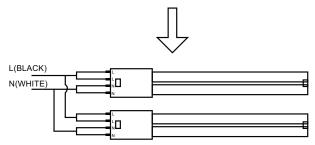
Rewire the fixture according to the wiring configuration
