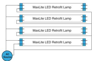
Note: These fixtures are for use only with lamps wired per the above example. Serious risk of electrocution, or fire if non-compatible lamp is installed.
