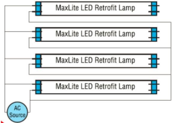
These fixtures are for use only with lamps wired per the above example. Serious risk of electrocution, or fire if non-compatible lamp is installed.
