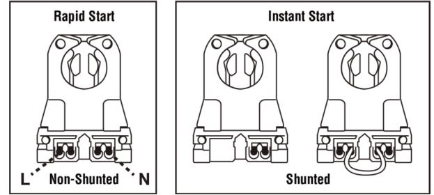
Figure 1. - Non-shunted & Shunted Lamp Holder
