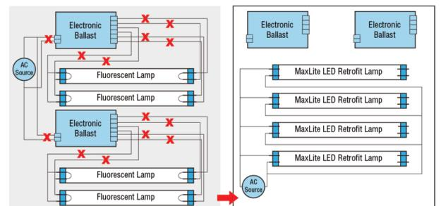
Figure 6. - Retrofit with Three/Four Lamps & Two Ballasts
