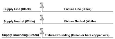
Wiring layout without photocell
