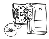
7. If you do not wish to use the photocell, unplug connector located at the top of fixture housing.
