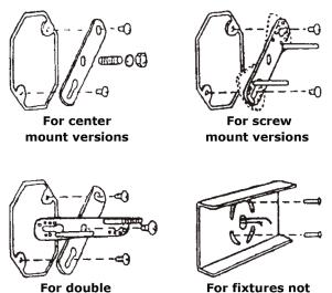
**3.)** Place cover over outlet box and secure. Mount glass.
