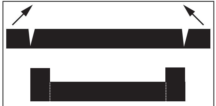
FIGURE 14. Form Air Seals into a U Shape
