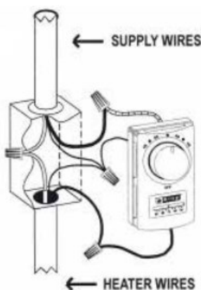
Connection Diagram for Wall Mounted Single Pole Thermostat
