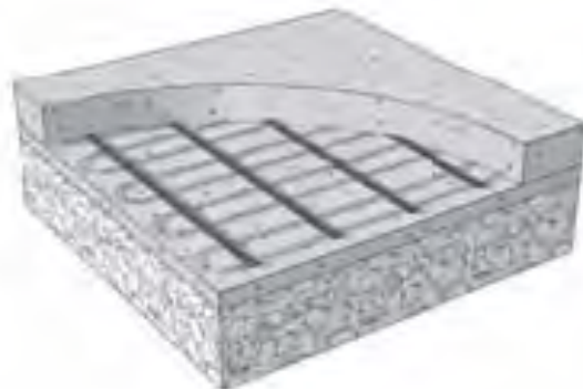
SC embedded in Asphalt
