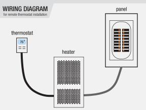
Power must be routed to heater first, then to remote thermostat.
