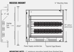
**MOUNTING NOTE:** 1" minimum mounting height from finished floor to allow clearance for the grill overlap.
