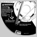
Push in the dashed area with a screwdriver to completely break tab.
