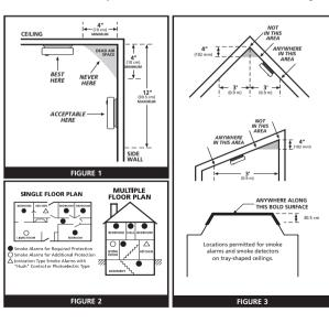
• NFPA 72 states: "Smoke alarms in rooms with ceiling slopes greater than 1 ft in 8 ft (.3m in 2.4 m) horizontally shall be located on the high side of the room." NFPA 72 states: "A row of detectors shall be spaced and located within 3 ft (0.9m) of the peak of the ceiling measured horizontally."
