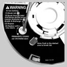
After the tab is broken, use the screwdriver to break through the label and turn the slotted arrow counter clockwise to the "PERMANENTLY DISABLE and DISCHARGE alarm" location. This will disable the alarm, stop the low battery "chirps" and render the alarm safe for disposal by draining the battery.
