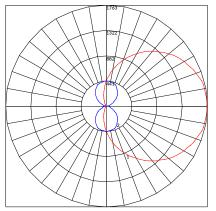
Maximum Candela = 1763 Located At Horizontal Angle = 90, Vertical Angle = 87.5 # 1 - Vertical Plane Through Horizontal Angles (90 - 270) (Through Max. Cd.) # 2 - Vertical Plane Through Horizontal Angles (0 - 180)
