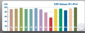
The CRISP SERIES DOWNLIGHT 18W lamp features a typical CRI the whole spectrum. Its exceptional R9-R14 values (R9 & R13) provide redder reds, natural looking skin tones and whiter whites. In addition, this lamp's color temperatures fall within a 4-step Macadam ellipse to ensure minimal color deviation across lamps.
