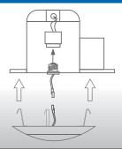
For use with the 14.5W CLICK downlight, these accessories allow for installation in a 4" recessed incandescent housing. Compatible with most standard 4" IC & Non-IC housings.
