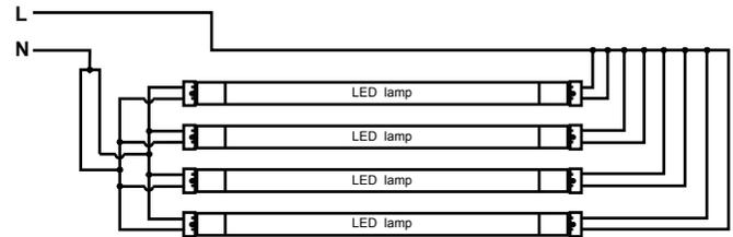
Step 2. Connect the lamps according to the above wiring diagram
