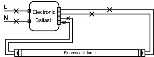
Step 1. Cut all wires connected to the existing ballast, remove the ballast.
