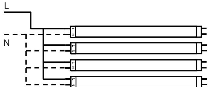
Step 1. Cut all wires connected to the existing ballast, remove the ballast.
