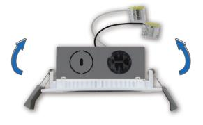
The 4" THINFIT SERIES DOWNLIGHT is designed to be used for both new construction and remodel installations. All wiring takes place inside the integrated J-box which features a pre-installed wire clamp, quick connects and an easily removable lid. After the downlight is wired, simply replace the lid and push the spring action clips into the ceiling cutout. Save time and materials with this easy to install downlight.
