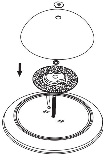
Slide the light engine center through the lamp pole screw.
