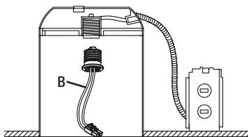
**4a** Installing into a recessed can: Screw the medium base (E26) socket adapter into the socket in the can.
