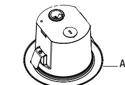
**6a** Insert the fixture into the can.
