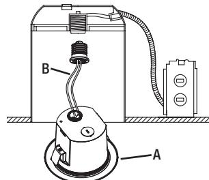
**5a** Plug the cable connector on the socket adapter into the fixture.
