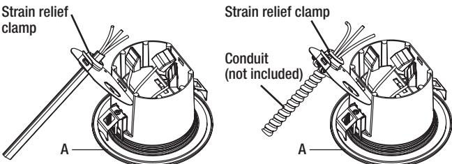
**4b** Run the wires based on local electrical code through the strain relief clamp and make the electrical connections. Insert the hot, neutral wires from the electrical source into the wire connectors of the black and white wires in the electrical box.
