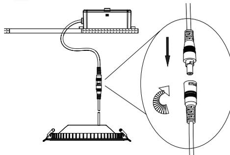
**9** Insert the electrical box into the opening in the ceiling. Connect the connector cable from the electrical box to the connector cable from the fixture.
