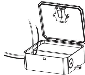
**7** Run wires per local electrical code and feed wires through the knock out hole.
