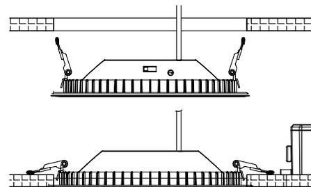
**10** Compress the spring clips and insert the fixture into the opening in the ceiling. Restore power at the electrical panel. Turn on the light switch to activate the fixture.
