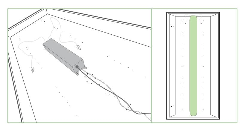
STEP 4: Once the ballast is removed replace it with the ESL Vision Quick Connect Driver. The driver is designed to fit in the same location as the previous ballast. Pull the DC lines to the end of the wire compartment. Replace the ballast cover.
