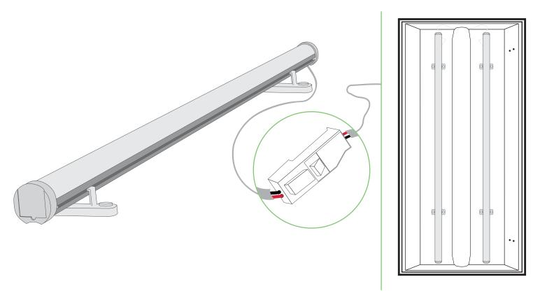
STEP 6: Clip Ti Tube into Ti Clips, connect the Quick Connects and push the wires back into the wire compartment.
