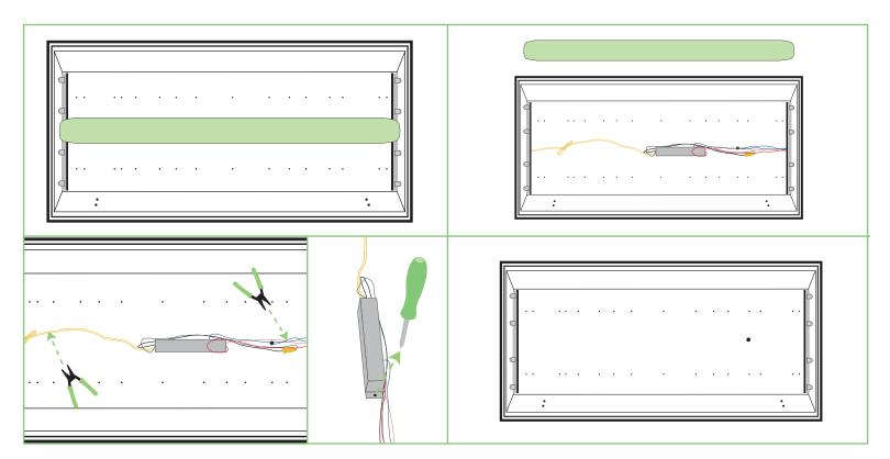
STEP 2: Once the lamps are removed, remove the wiring compartment and disconnect the ballast.
