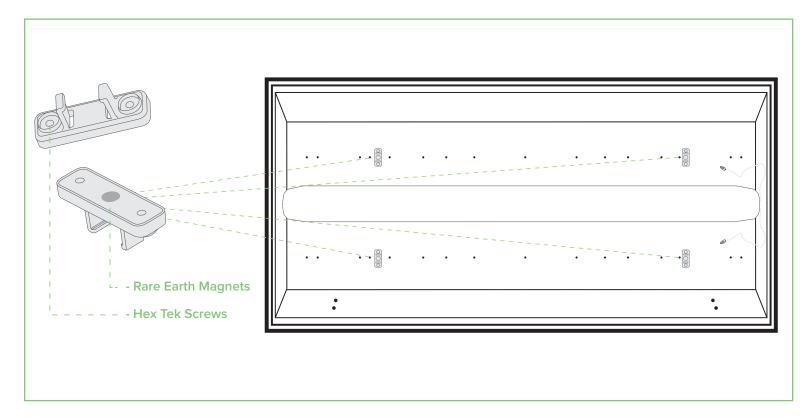
STEP 5: Place Ti Clips into position. Ti Clips have strong magnets on the back. This allows the clips to be repositionable for perfect easy and pefect palcement. Once the clips are in the desired position, screw them into the fixture using the provided. Hex Tek Screw.
