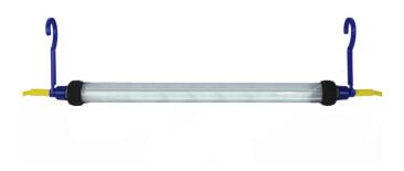
• High impact, shatter-proof tube with replaceable frosted tube shield• Beam angle available in 200° and 360°• Bi-directional version offers glare protection to prevent eye strain• Wired with 15A, 125V, water-tight plug & feed-thru water-tight connector• Driver range of 100-277 volts at 50/60 Hz• Environmental rating: Suitable for outdoor use in wet locations
