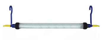
• High impact, shatter-proof tube with replaceable frosted tube shield• Beam angle available in 200° and 360°• Bi-directional version offers glare protection to prevent eye strain• Wired with 15A, 125V, water-tight plug & feed-thru water-tight connector• Driver range of 100-277 volts at 50/60 Hz• Environmental rating: Suitable for outdoor use in wet locations
