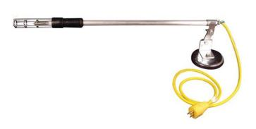
• Extra Bright, 500-w Tungsten Lamp• 120V, 8800 Lumens• N5-15 Industrial Water-tight Plug with 5' SOW Cord• Designed to fit through Boiler Inspection opening – 1.8" diameter• Curved handle version for directing light where you need it• Grounded Handle• Magnetic Mount for Stability• Welded Steel Cage to Protect Lamp• Replacement Parts Available
