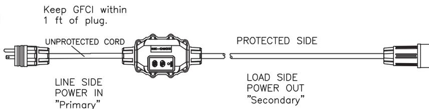
OSHA and the NEC call for the use of GFCIs in all 125 volt 15,20 and 30 amp circuits. Consult your local safety codes for additional GFCI use regulations.
