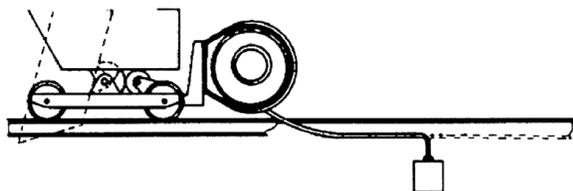
The reel needs to pickup ("retrieve") the cable. The reel is mounted on moving equipment. Cable is pulled out by machine.
