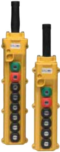
The 5500 Series uses sets of two buttons to build ever increasing sized stations. From 2 button to 12 button pendants, this series is the work horse of the 5500 Series. The design is more rugged than the 5500-PG series with rubber button boots and housing seals. NEMA 4X rated, these pendants can be used outdoors with confidence. With a wide variety of switches and controls that can be installed, this series is the best of rugged design and economically priced pendants.
