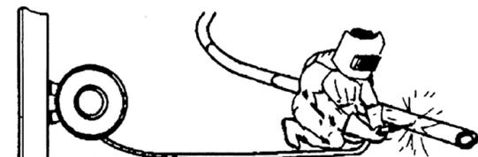
The reel needs to "drag" the cable through supports or along the ground horizontally. The reel is usually stationary. Cable can be pulled out by hand or by machine. Note: This application is the hardest on cable life.
