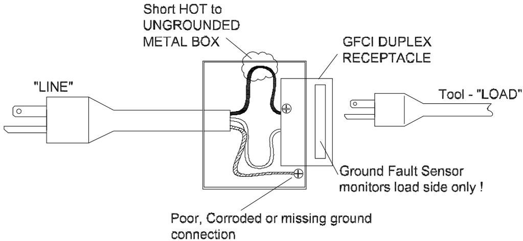
As the diagram shows, the metal gang box can have a common situation in which the earth ground is poor or not connected. There can be a hot short to the metal box in which you now have a "hot" box. The short will not trip the circuit breaker nor will the GFCI trip. The GFCI sensor only watches the "load" side of the receptacle, not the line side. The GFCI is worthless in this situation.
