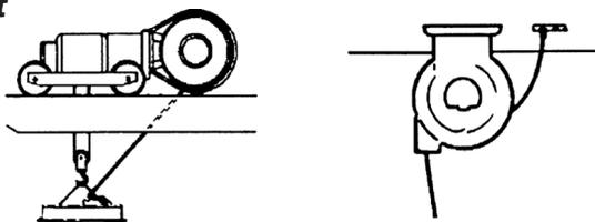
The reel needs to "lift" the cable vertically. The reel is usually stationary. Cable is pulled out of the reel by machine or by hand (as with an overhead light source or a pendant station.)
