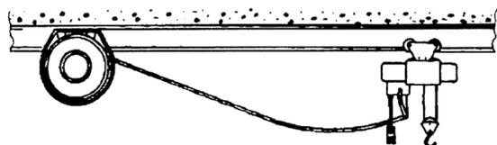
The cable is "stretched" horizontally and is unsupported. The reel may be stationary mounted or mounted onto moving equipment. Cable is pulled out by machine. An extra 6% -10% in cable beyond active travel is required for cable sag.
