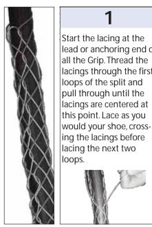
Start the lacing at the lead or anchoring end of all the Grip. Thread the lacings through the first loops of the split and pull through until the lacings are centered at
