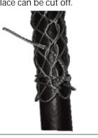
Split Grips, closed with a rod, eliminate the time and guesswork of on-the-job lacing. The stainless steel rod is a precise built-in feature which makes threading easy and fast. The strands of the mesh pass around the rod and match up with the strands from the opposite direction. The rod does not touch the cable at any point and therefore cannot cut the cable. Rod Closing Grips are salvageable; may be removed and reused as many times as desired.
