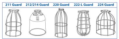
**Note:** Add "-P" to part number to indicate vinyl coated, grounded wire. 214 has a 1-3/4" diameter collar • 212 has a 1-1/2" diameter collar.
