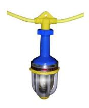
• cETLus listed• Class I & II Div 1 & 2, Groups C, D, F & G• NEMA 4X Rated, and Wet location rated• Copper-free, cast aluminum, anti-spark guard• High-impact tempered borosilicate glass globe • Heat, chemical and impact resistant, glass reinforced handle• Cord restraint seal system provides flex and water resistance• Accommodates #16/3 to #14/3 in various types of cord jackets• Stringlights are available in 65' and 100 ft. cord lengths• -20°C to 40°C Ambient
