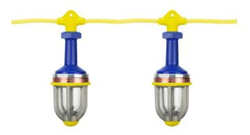
• cETLus listed• Class I & II Div 1 & 2, Groups C, D, F & G• NEMA 4X Rated, and Wet location rated• Copper-free, cast aluminum, anti-spark guard• High-impact tempered borosilicate glass globe • Heat, chemical and impact resistant, glass reinforced handle• Cord restraint seal system provides flex and water resistance• Accommodates #16/3 to #14/3 in various types of cord jackets• Stringlights are available in 65' and 100 ft. cord lengths• -20°C to 40°C Ambient
