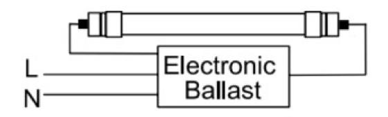
Type B (AC directly, double end ballast bypass) Assembly introduction:
